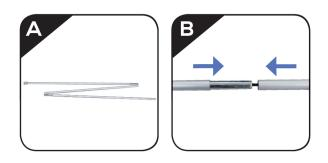
**Step 3**Insert telescopic pole into hole.
